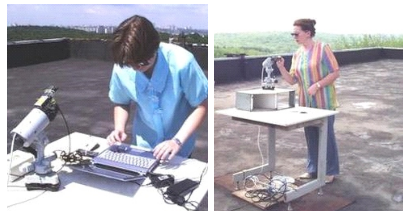
Dr. T.Orlova and Prof. I.Terenetskaya adjust the UV measuring device 'D-dosimeter'.
